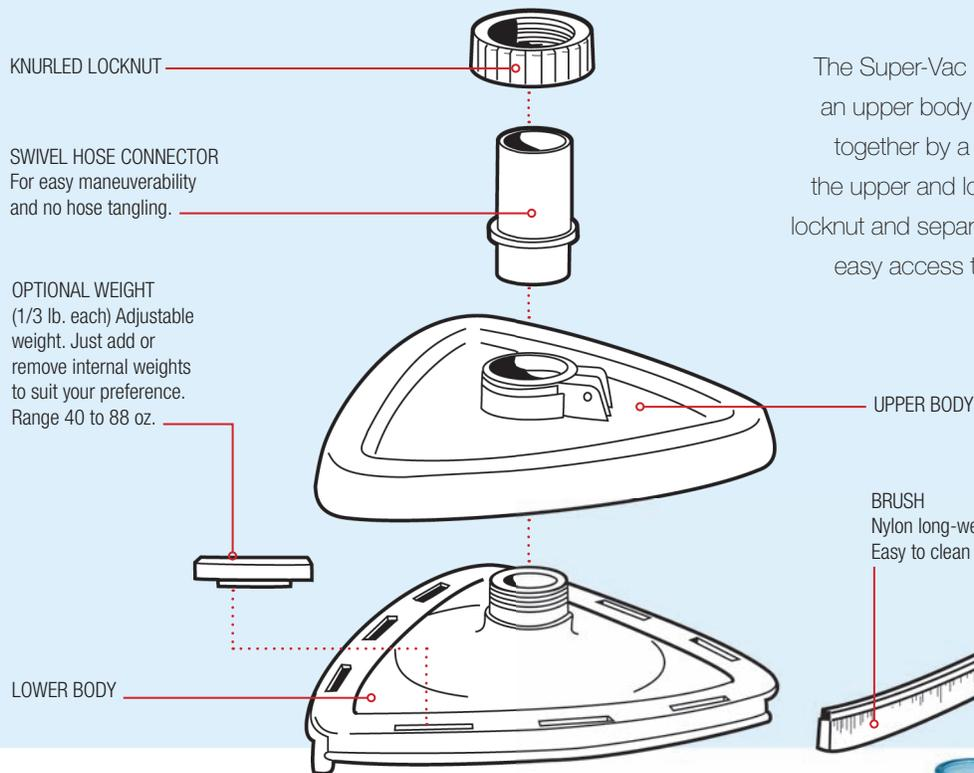
The Super-Vac is designed in two main parts — an upper body and lower body. They are joined together by a knurled locknut. To disassemble the upper and lower bodies, simply unscrew the locknut and separate the two parts. This allows for easy access to brushes and optional weights.
